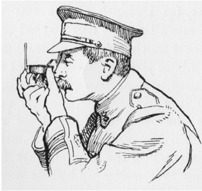
5.2 Use of prismatic compass, from Mockler-Ferryman
